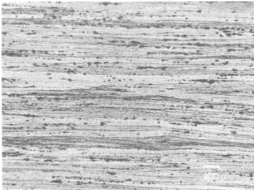
Figure 1 Polished and etched section of 7017-T651 plate perpendicular to rolling plane revealing highly banded structure with inclusions. The rolling direction is from left to right.
